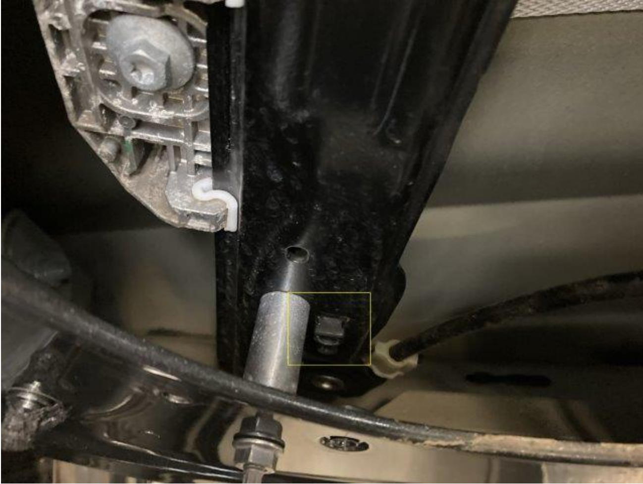
Figure 15. Checking end stop of door window.
