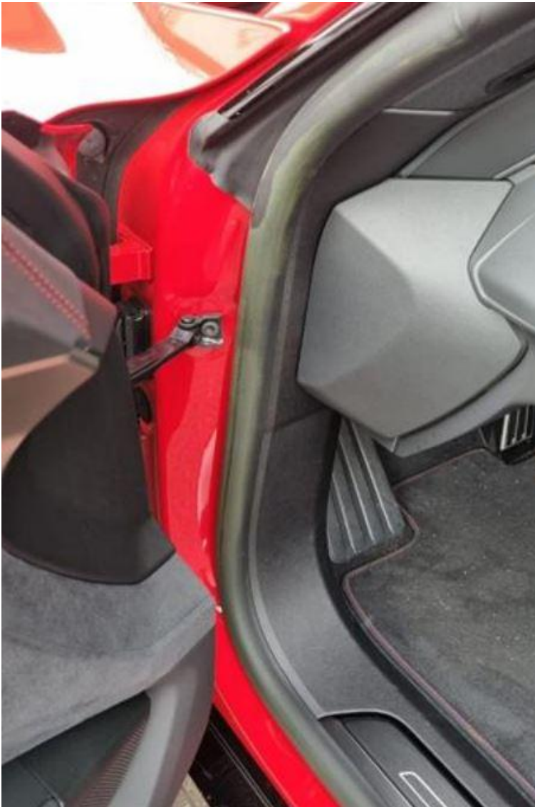
Figure 1: Door seal discolored green (example photo).
