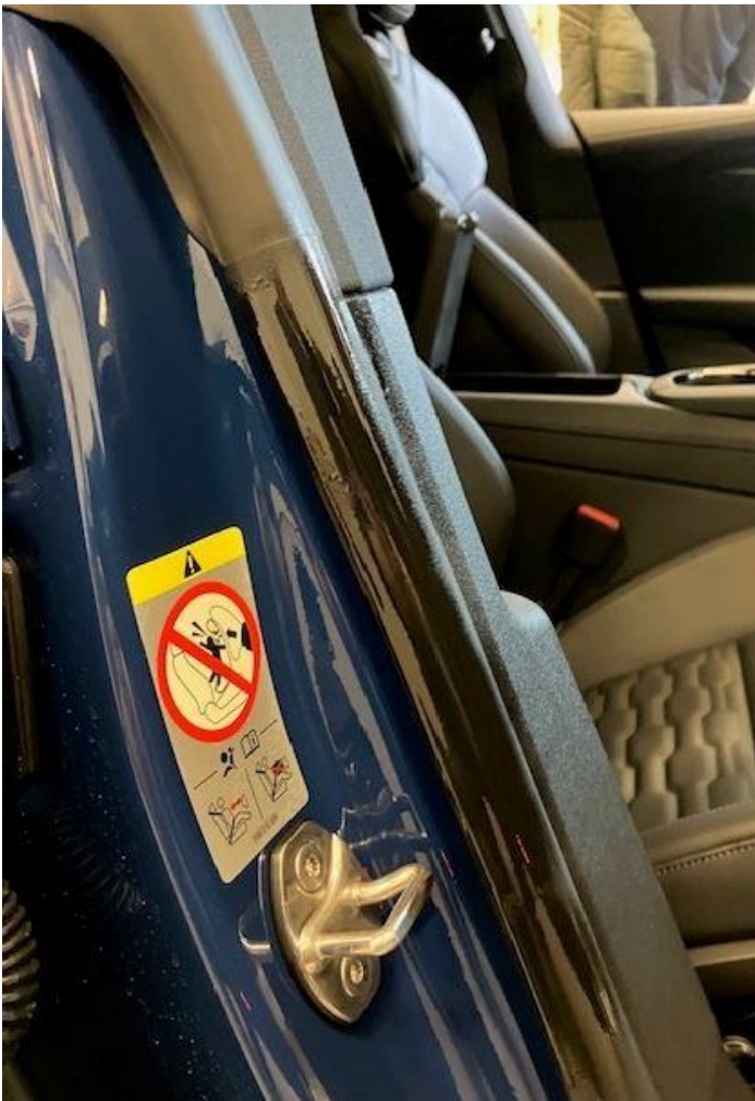
Figure 3. Discolored door seal coated with cleaning solution.
