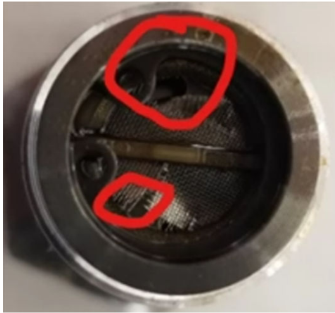
Fig. 2 OCV Filter Torn
