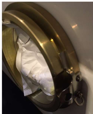
Figure 12: Desiccant Bags to be Removed
