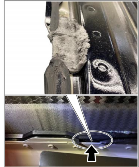
Bonding on roof module
