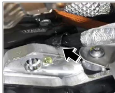
Friction welded joint for ATF cooling line PHEV faulty
