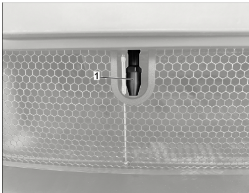
Assembly of front lip rods
