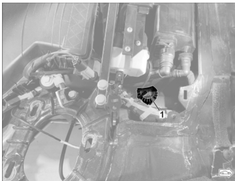
Installing front left resistor
