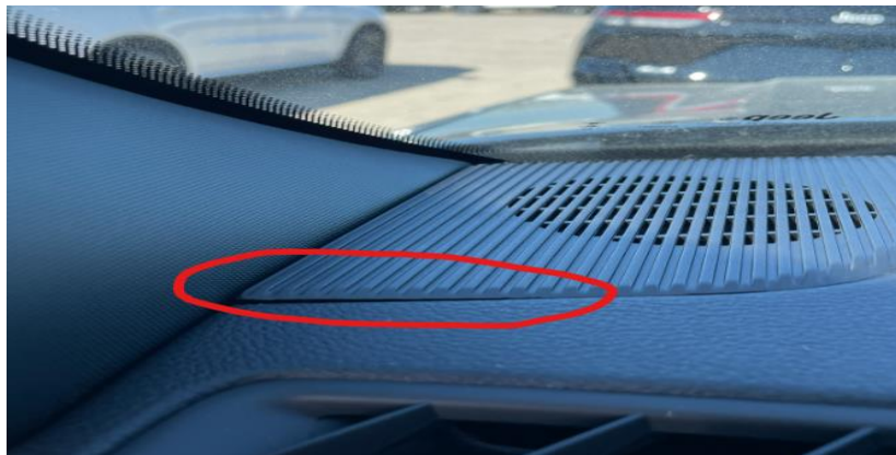
Fig 2 Gap In Corner(s) Of Grille.
