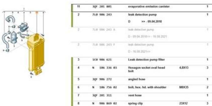
Figure 1. Example: ETKA indicates that the EVAP Canister is available as a separate component within the complete assembly.
