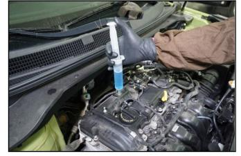
5. Using **SST 09580 3D100** pressurize each cylinder under pneumatic pressure (2~3 bar) for three (3) minutes.
