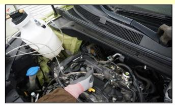
9. Place a clean towel/shop rag over the spark holes. Crank the engine for 3-5 seconds, 3 times.
