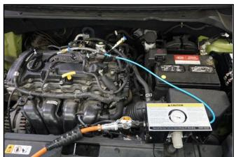
6a. Connect the four (4) hoses & adaptors to each cylinder as shown.
