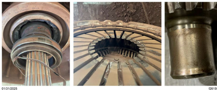
Fig. 2, Examples of CPCA, Clutch, and Input Shaft Wear
