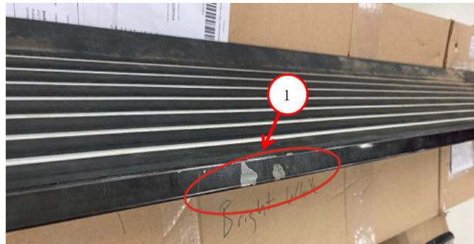
Fig. 1 Paint Peeling Example
