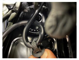
3. The harness is held to the back of the seat frame with a push-in clip. You can move this clip on the wiring harness, or move the harness around to introduce more slack.
