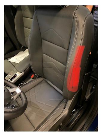
1. Check the resistance of the seat-mounted air bag before seat disassembly.
