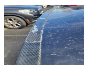
The clear coat on the carbon fiber M Performance rear spoiler is delaminating.
