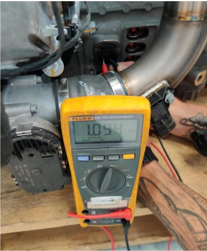
Stator winding thermistor resistance at ambient temperature pins 12 & 13
