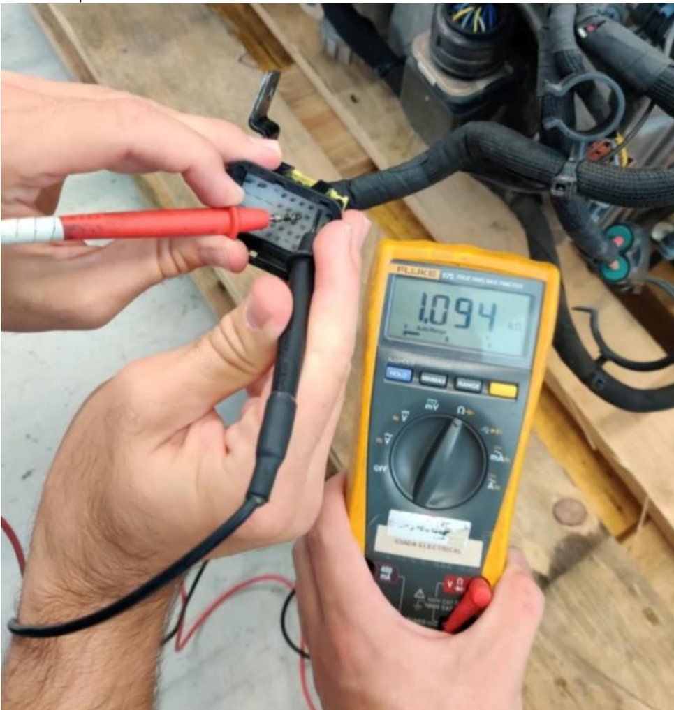
Stator winding temperature thermistor checks at the transmission in-line connector pins 24 & 33
