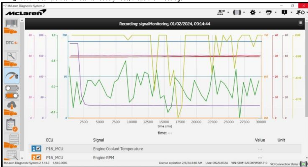
Diagram shows temperature at 180°C dropping to 40°C (Purple Trace)
