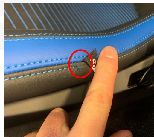
Damage of stitchings
