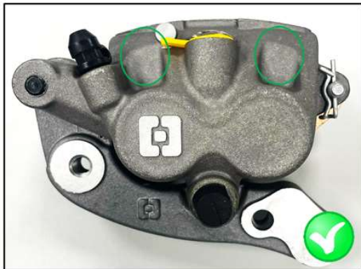
Figure 3: Front Brake caliper from OK sub-supplier 1 Calipers that look like this do not need replaced.
