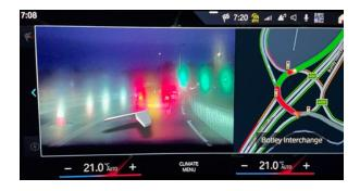
The Augmented Reality Camera (ARCAM) shows up blurry when activated.
