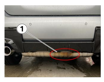
Tarnishing of the metal (1) on the rear silencer is caused by the heating and cooling of the exhaust.
