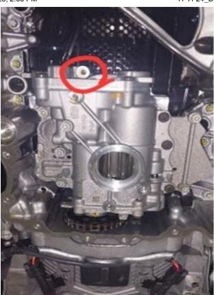
2. Tighten the screw on oil pump to 8.4 Nm. For the circle in the photo, the oil pump pickup has been removed for clarity.
