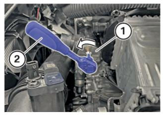
Cylinder 6 intermediate lever may interfere when trying to install the intake camshaft timing tools.
