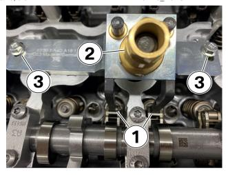
Special tool 83 30 5 A4D A18 must aligned properly with the rollers (1).
