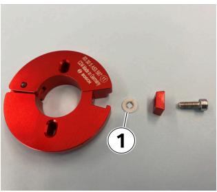
Tool 83 30 5 A53 587 may bind when removing it from both of the VANOS adjusters, the plastic washer (1) may be binding the tool and will not allow it to collapse when the screw is loosened.
