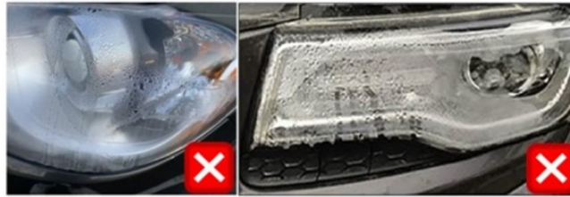
Fig. 3 Condensation/Fogging Not Beginning To Clear Examples
