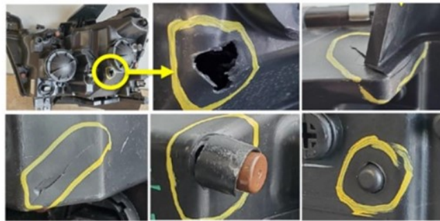
Fig. 4 Cracked, Damaged Or Broken Headlamp Examples
