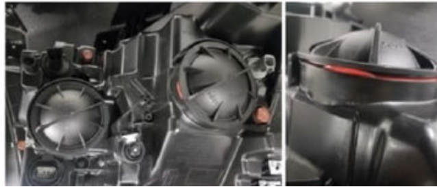
Fig. 6 Incorrectly Installed Access Caps Examples
