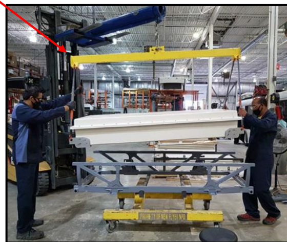
Figure 5: Upper ESS Assembly Removal Location Reference.
