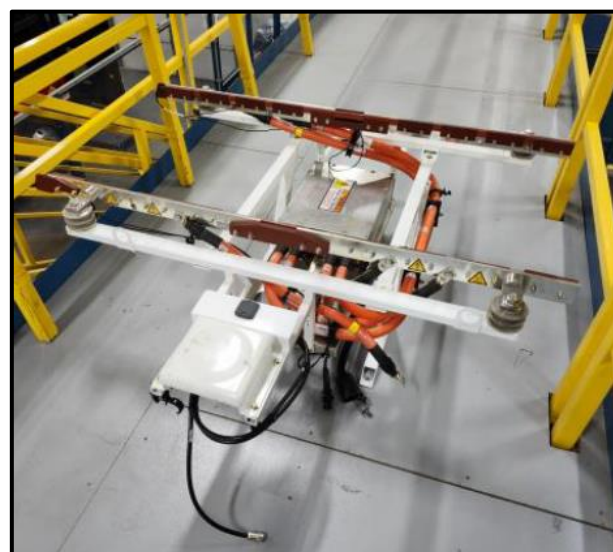
Figure 3C: Charge Rail Removal Location Reference.
