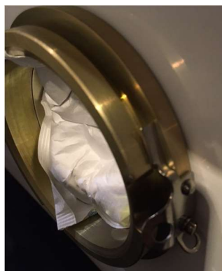
Figure 12: Desiccant Bags to be Removed
