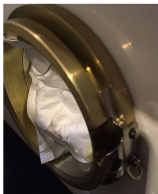
Figure 12: Desiccant Bags to be Removed
