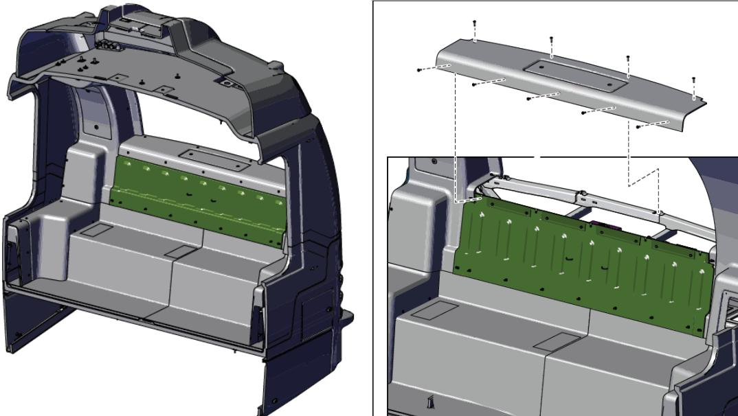
3. Locate the existing Bendix ABS ECU at the streetside rear corner of the rear deck plate.
