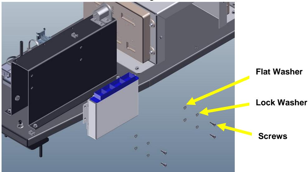
9. Using a Torque Driver, **torque each of the four Socket Head Cap Screws to 44 in-lb.**
