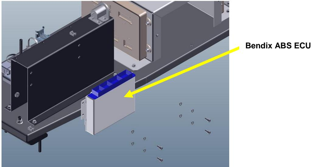
6. Place the removed ABS ECU aside for return to Proterra/Bendix.
