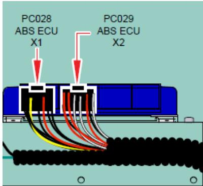
5. Using a 4mm Allen bit socket (or Allen wrench), remove the four (4) screws, lock washers, and flat washers that secure the ABS ECU to the vertical bracket on the rear deck plate.
