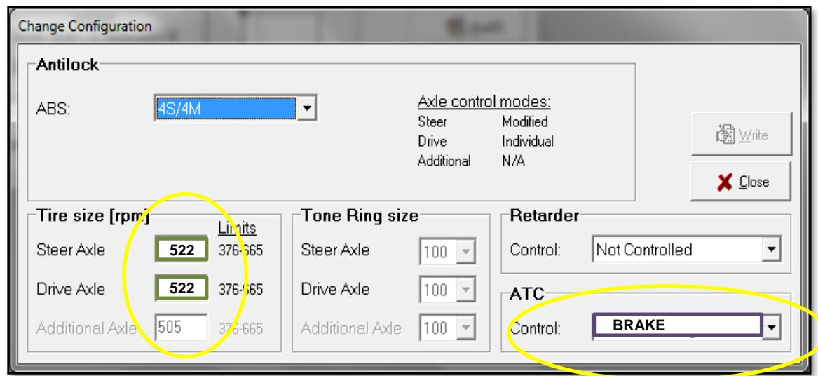
18. Verify the configuration has the appropriate settings for the vehicle in question. When these settings have been changed, select “Write” option.
