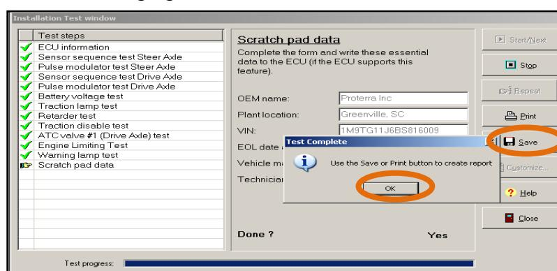
33. Keep a copy of these ABS configuration records. It should be printed off or saved.
