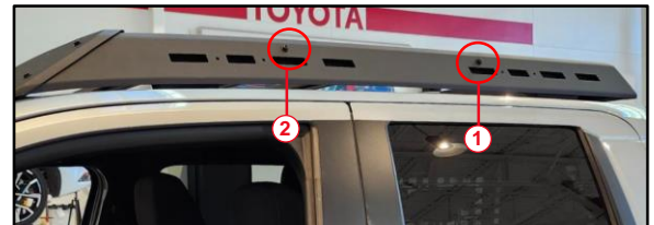
Figure 7. Roof Rack Side Panel Hardware
