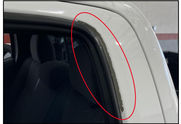
Figure 1. Paint Peeling on Door Frame
