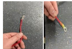
FIGURE 1. BEFORE (LEFT) & AFTER (RIGHT) ADDING RING TERMINAL
