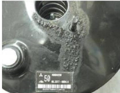
Damage caused by brake fluid
