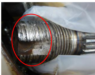
Damaged axle shaft
