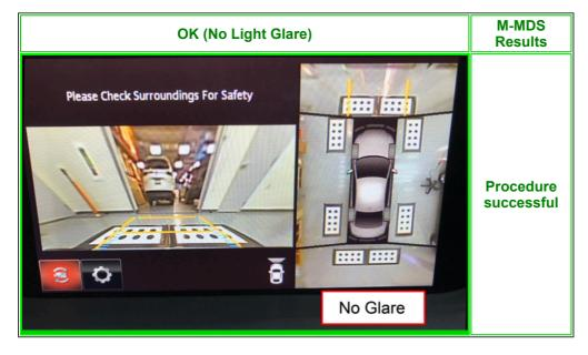
If light glare is found using the center display, remove the light glare.
