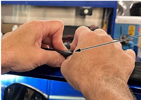
Pinch to aid in placing edges into the channel.
