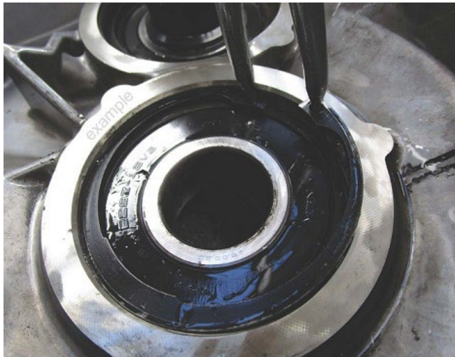
Figure 9. Removing retaining ring (example).
