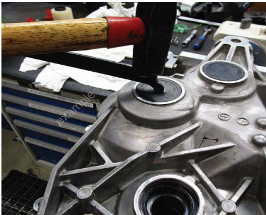
Figure 2. Removing filler cap with extractor lever -VW681- (example).
