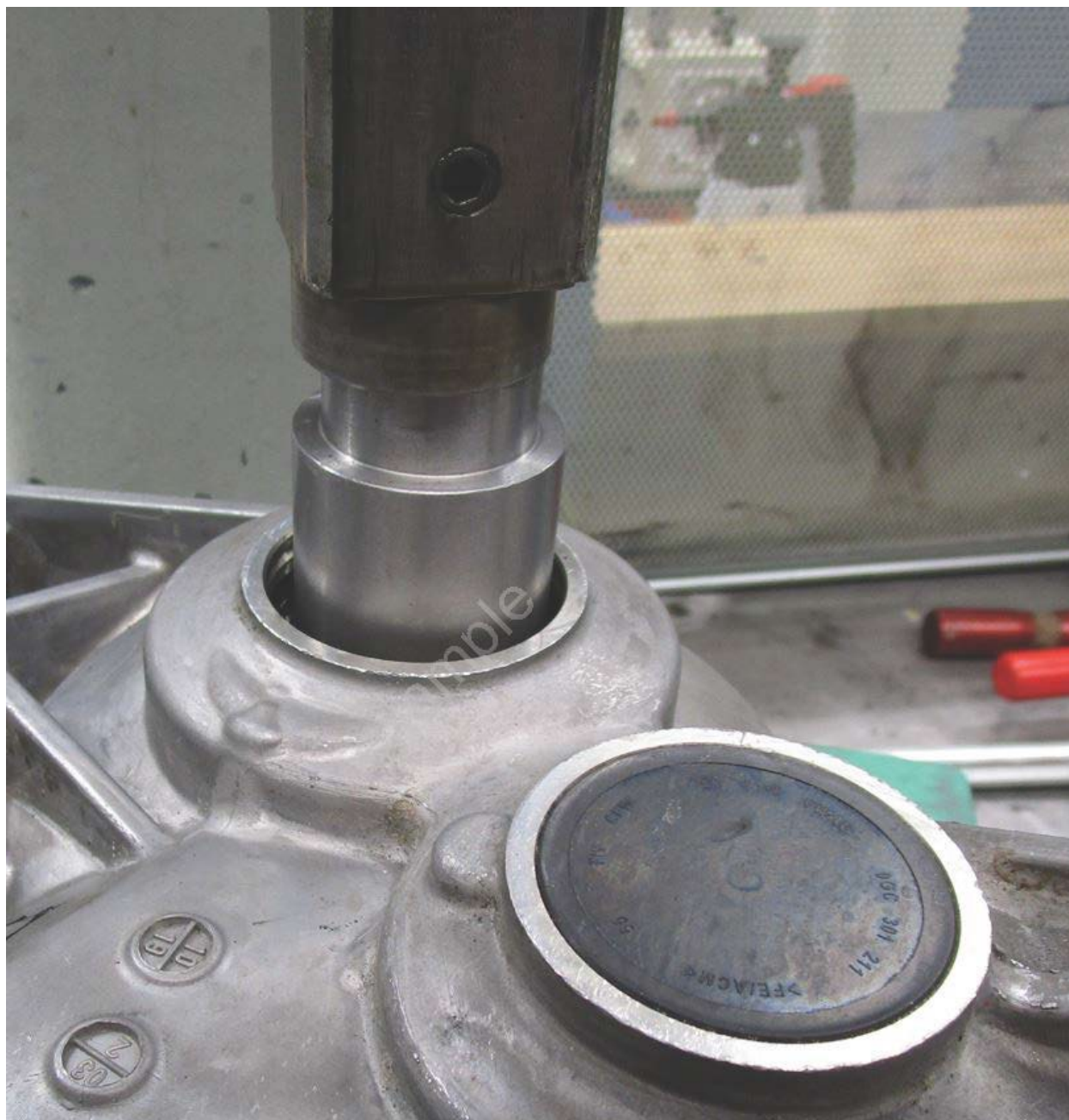
Figure 10. Pressing out bearing for intermediate shaft (example).
