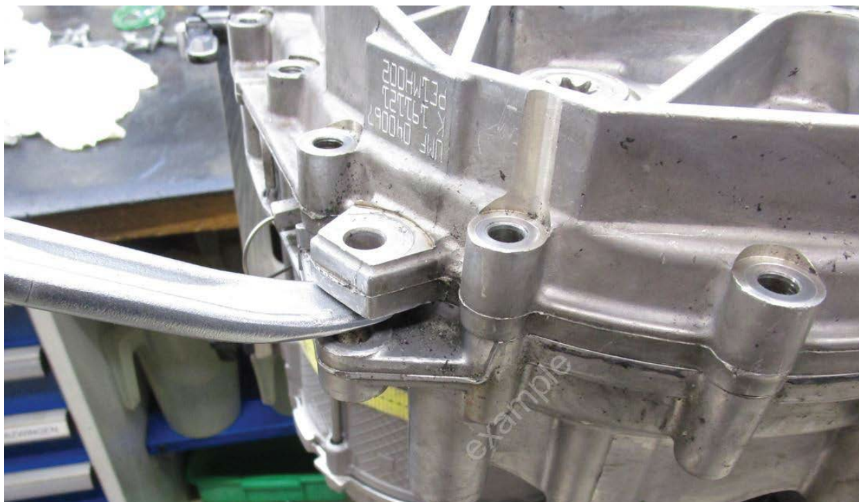
Figure 6. Separating sections of gearbox housing from each other using assembly lever.
