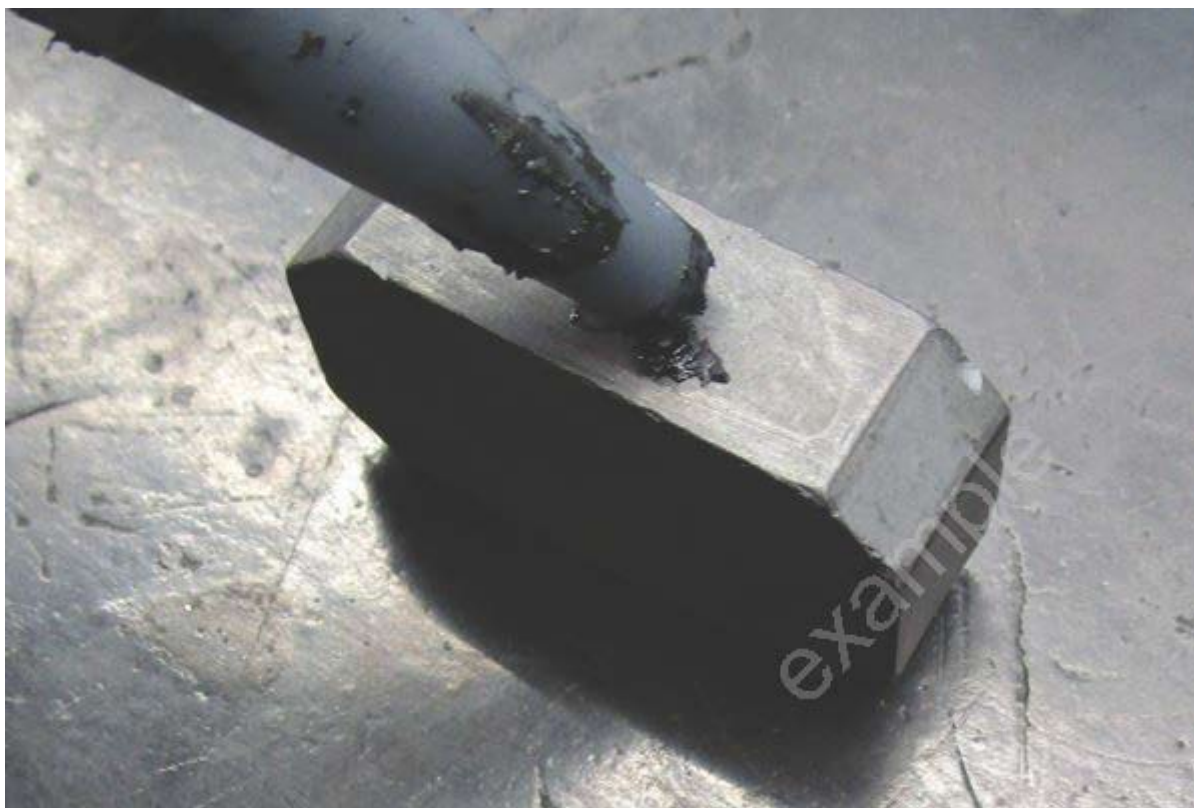
Figure 18. Magnet with silicone sealant (example).
