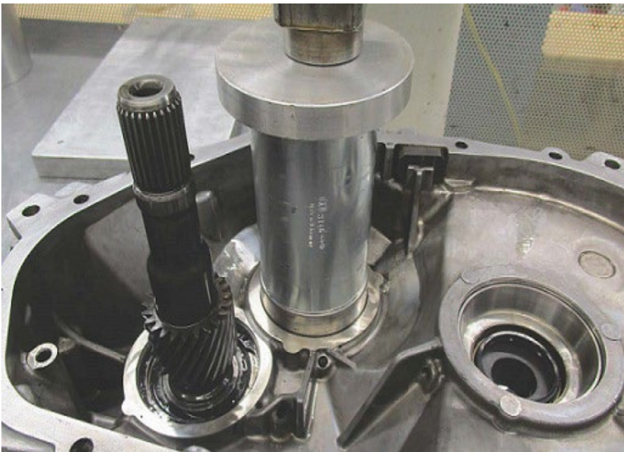
Figure 14. Pressing in new bearing for intermediate shaft with tube -3146-.
