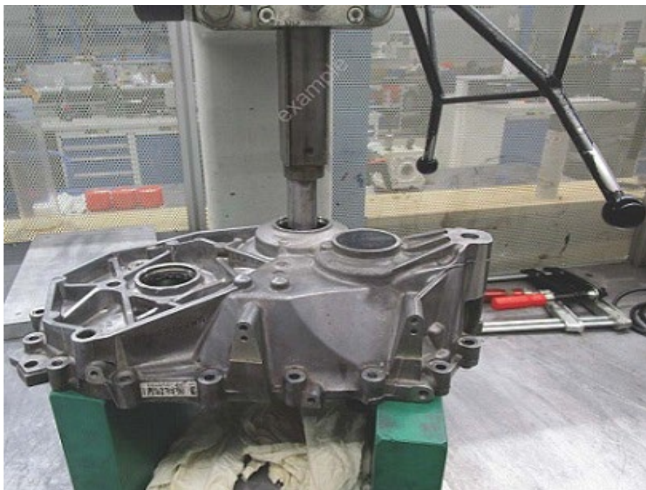
Figure 8. Pressing out intermediate shaft (example).
