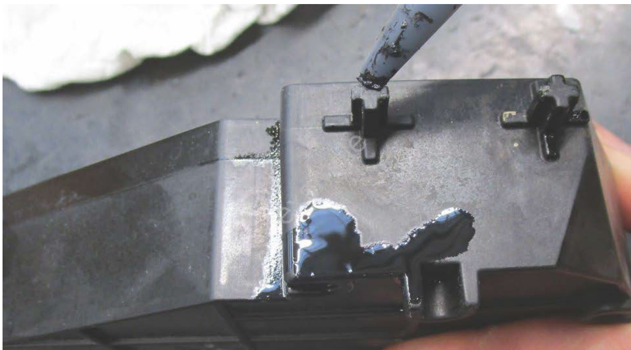
Figure 20. Lightly applying silicone sealant to attachment point (example).
