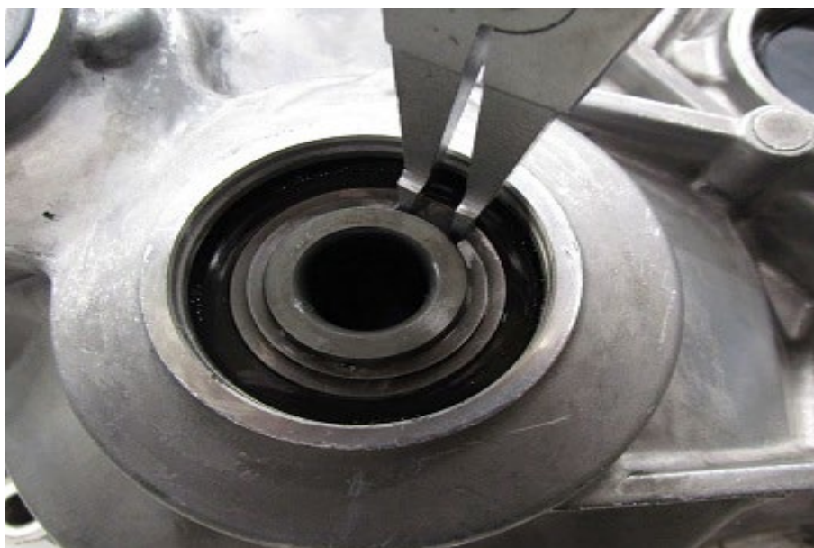
Figure 3. Removing retaining ring for inner ring of intermediate shaft (example).
