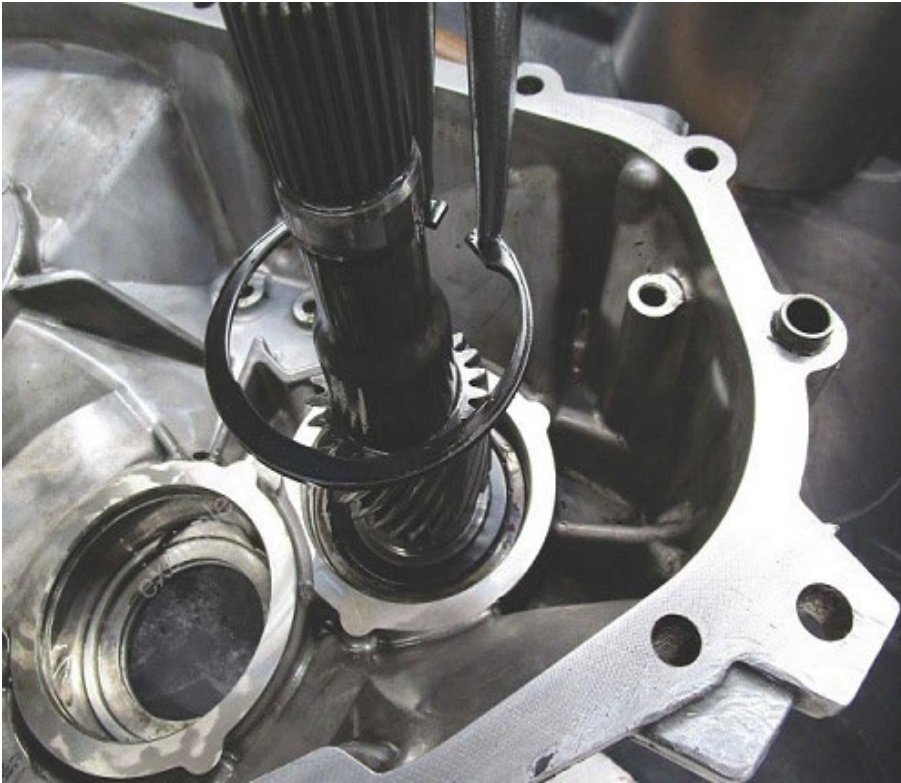
Figure 11. Removing outer retaining ring for drive shaft (example).
