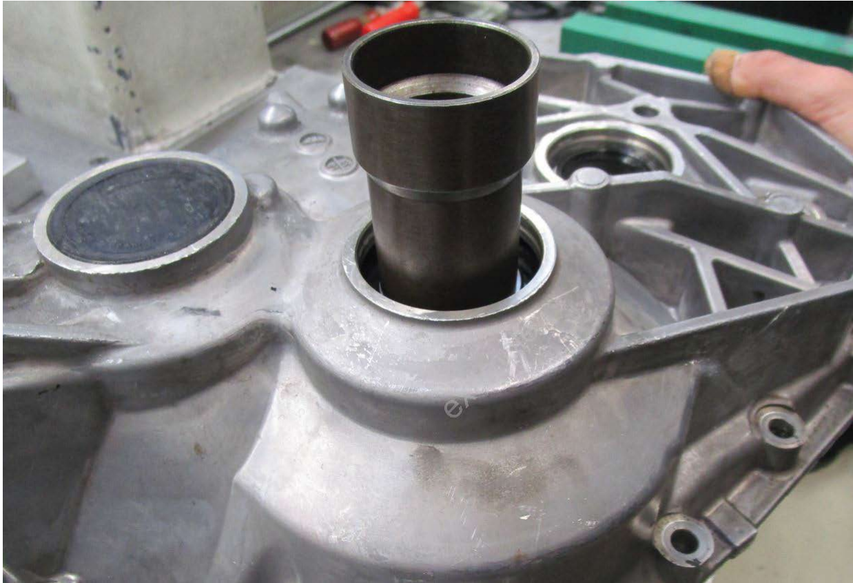
Figure 16. Supporting inner ring with thrust piece -VW454- (example).
