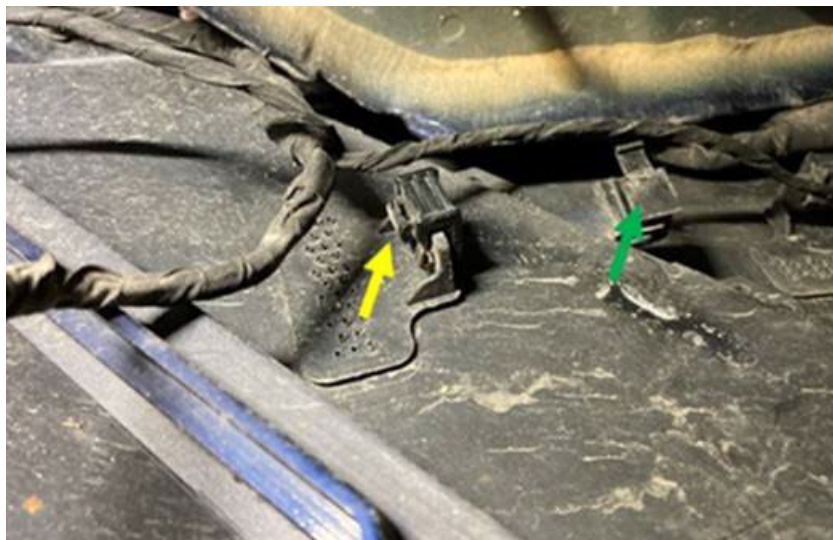
Figure 2: Cable ties to be removed.
