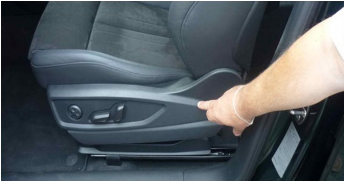
Figure 1. Noise from the seat height adjuster.
