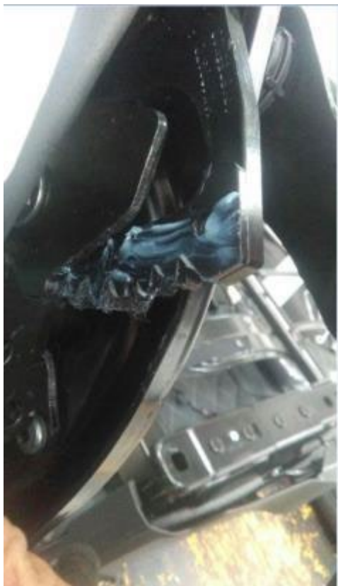
Figure 3. Grease applied to the toothed segment and the lateral surfaces.
