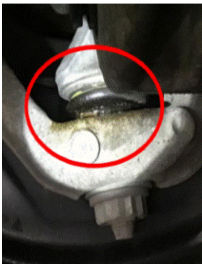
Figure 1: Grease emerging from swivel joint.
