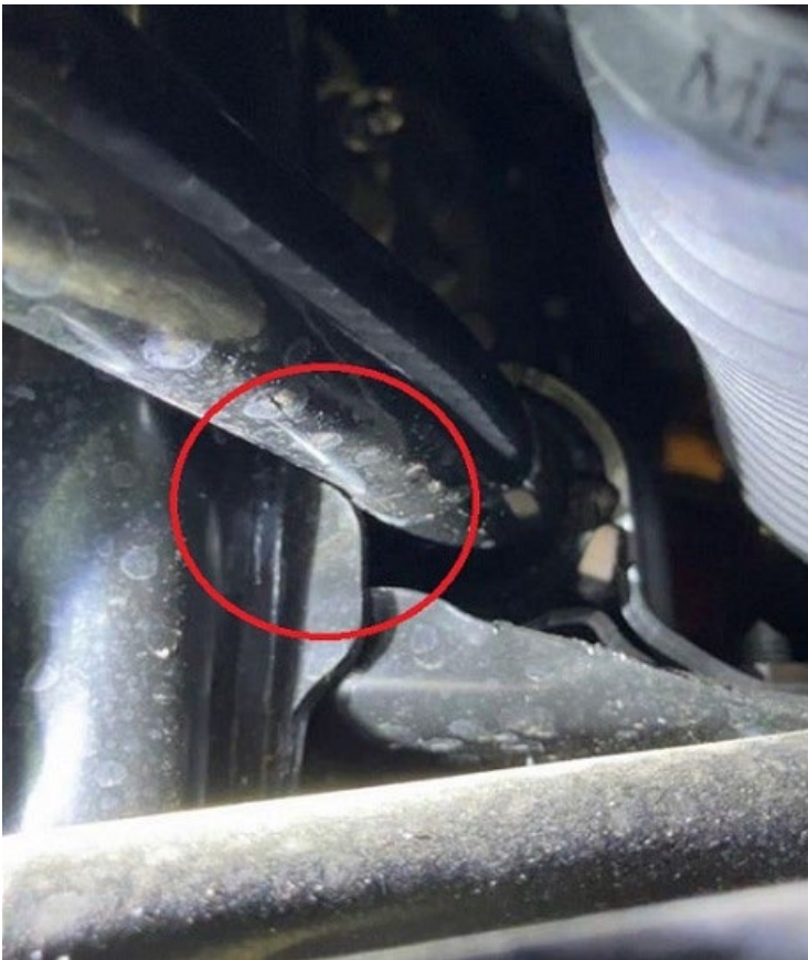
Figure 2. The anti-roll bar rests against the subframe of the front axle.
