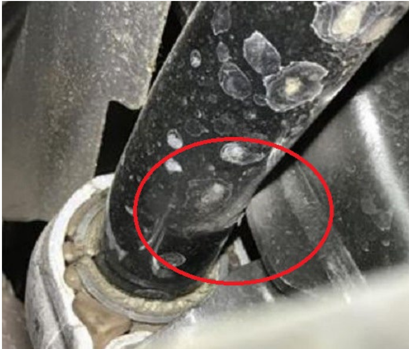
Figure 1. The anti-roll bar rests against the subframe of the front axle.
