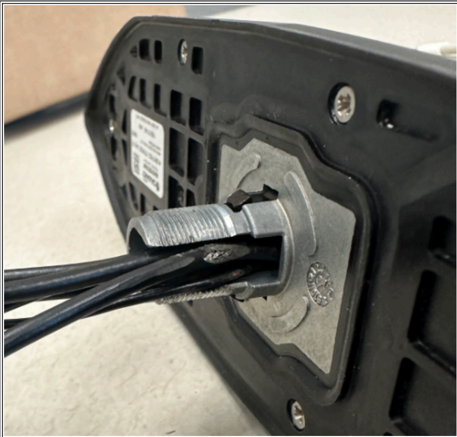
Figure 2: Damaged Antenna Cables
