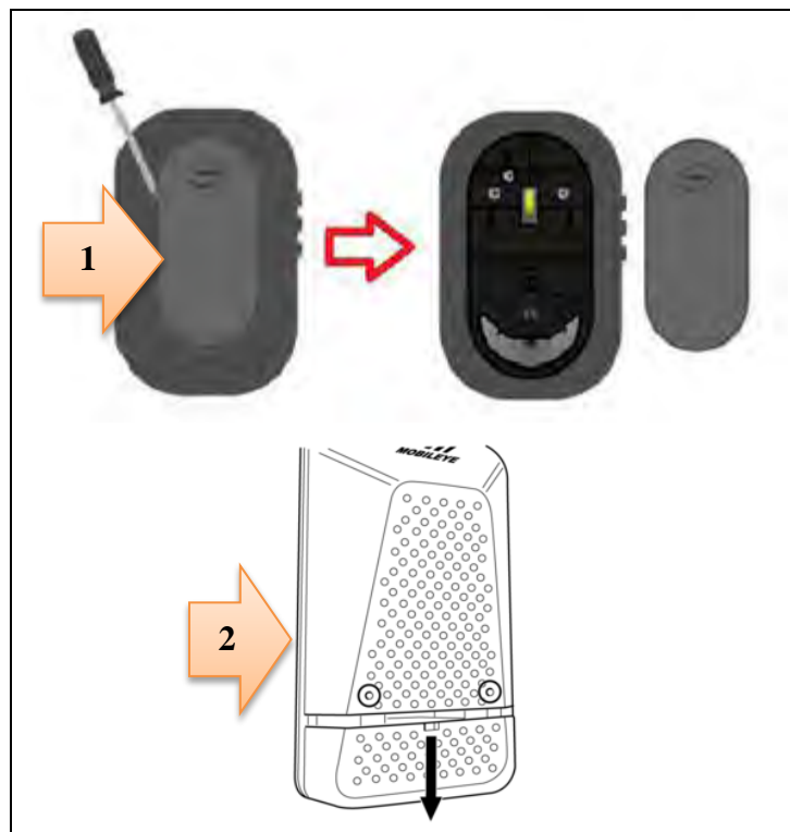
Figure 58 1. Mobileye 8: Remove oval cover. 2. Mobileye 6: Remove rectangular cover.
