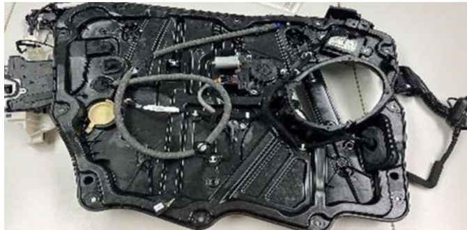
Fig. 26 Carrier Plate Wet Side Facing Down
