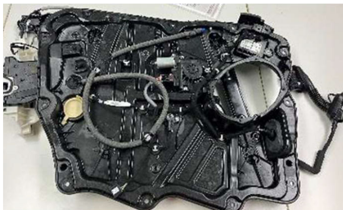
Fig. 9 Carrier Plate Wet Side Facing Down
