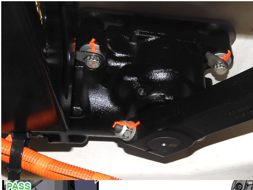
Example of a Good Unbroken Torque Stripe. The torque stripe is intact.
