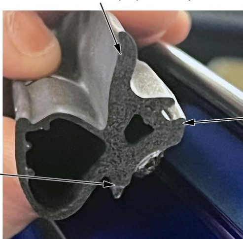
LOWER EDGE Ensure lower edge is inside channel.
