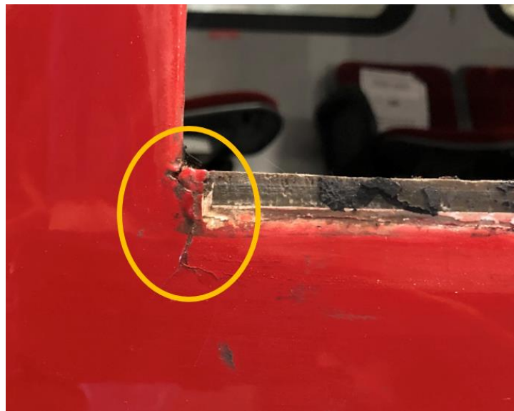
Figure 1 Example of rear door corner crack
