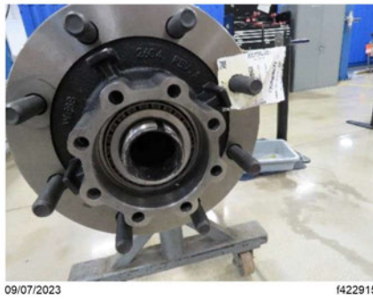
Fig. 4, Spindle Nut Removal
