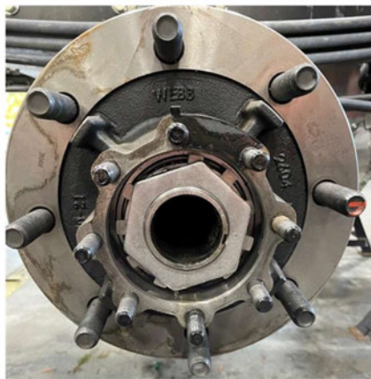
Fig. 3, Outer Jam Nut Removal
