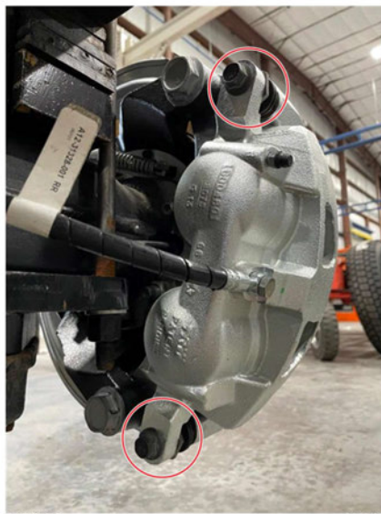
Fig. 1, Brake Caliper Mounting Bolts Removal
