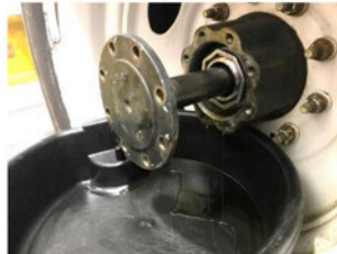
Fig. 2, Drain Pan Under the Axle Shaft Flange
