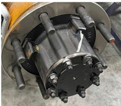
Fig. 12, Positioning the Axle into the Wheel End
