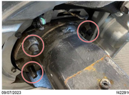
Fig. 5, Nuts to be Removed
