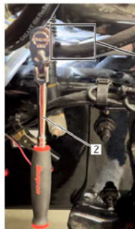
Fig. 3, Location of the Bolt to Adjust the Coolant Pipe Position
