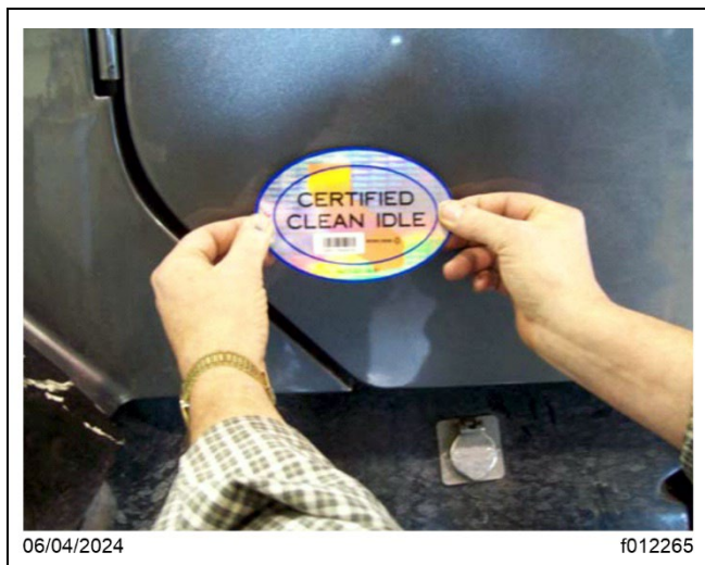
Fig. 3, Placing New Label
