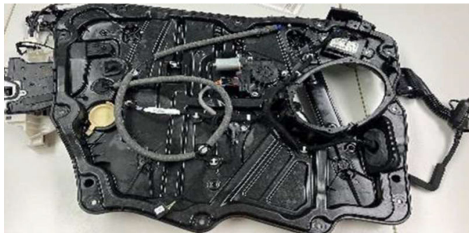
Fig. 26 Carrier Plate Wet Side Facing Down
