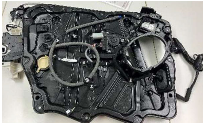
Fig. 9 Carrier Plate Wet Side Facing Down
