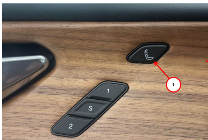
Fig. 1 Front Left Door Panel Seat Massage Switch
