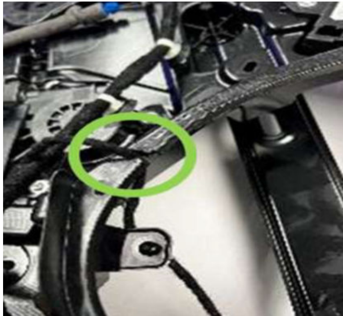
Fig. 22 Speaker Wire Retaining Clip
