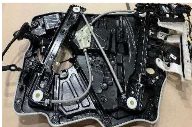
Fig. 39 Carrier Plate Dry Side Facing Down
