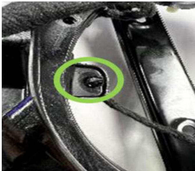
Fig. 23 Speaker Wire Harness Backside Clip
