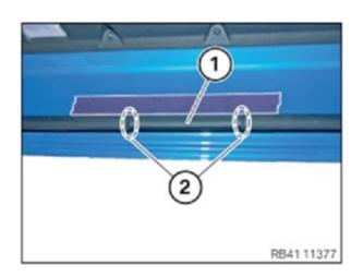
2. For these cases, where the main door seal detaches in the area that it is not visible to the customer (shown above), repair the detached portion of the main door seal by replacing the affected section by following the repair instructions listed in ISTA/AIR 51 71 003.
