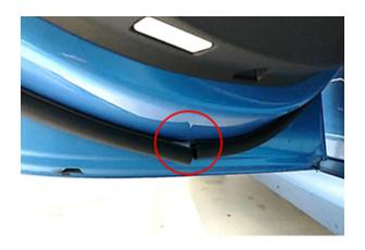
On the main door seal, detachment behavior can be detected in the sealing joint area.
