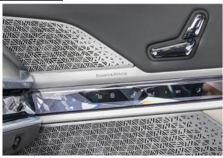
After the vehicle has been programmed with either RSU (Remote Software Update) or ISTA (I-Level 24-07-5xx), the ambient light on the door panel speakers will only illuminate in white.
