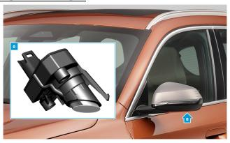
Replace the light module in the affected exterior mirror assembly.
